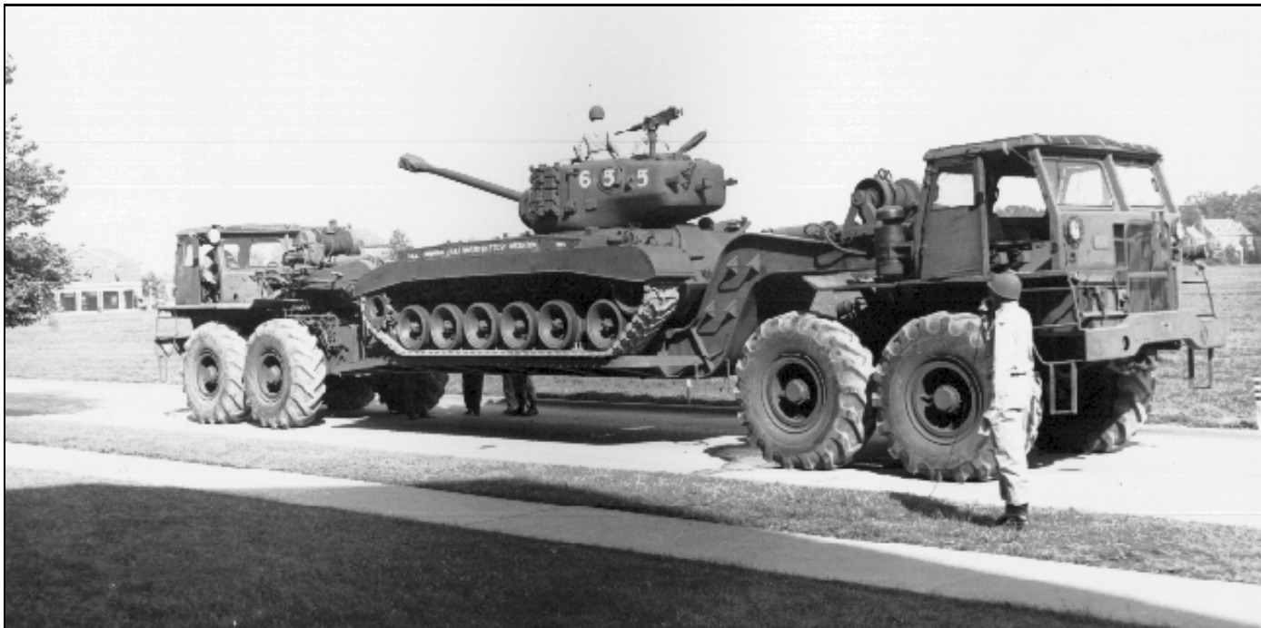
The M-26 tank, seen here on an M8 tank transporter, did not enter combat in the European Theater until the final days of WWII. Its armor protection, 90mm gun, and modern torsion bar suspension finally put U.S. tankers on a par with their German opponents.
